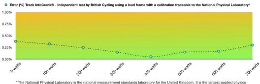
Tests are also conducted well above the normal operating range of a rider in order to validate the instantaneous torque numbers that might be achieved during a sprint or standing start. As the graph below shows, the error is remarkably steady at all torque levels.
